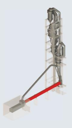
With the increasing demands set for energy consumption and CO2 emissions from cement plants, and the potential of significantly lowered maintenance costs, Skamol has developed the SkamoCeramic M-Extra insulating brick. It has proven very efficient as back up insulation in duallining solutions in rotary kilns:
