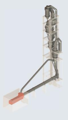
In cement clinker coolers and kiln hoods, dense refractory linings backed by insulation materials often result in an unnecessarily heavy construction.
