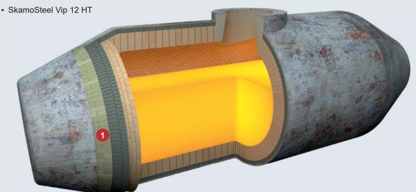
The transportation of hot metal constitutes one of the most important steps of the production chain in the iron and steel industry – a step that is made more complex by resisting the re-oxidization of the hot metal, securing both a high, stable temperature, and the structural integrity of the refractory lining.
