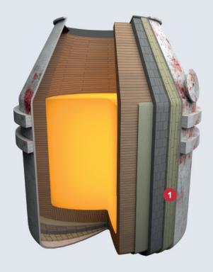
To protect the steel shell of the converter and prolong the lifetime of the entire application, the converter is lined with refractory and insulating materials. The preferred insulating materials must be able to resist the high intermediate temperatures in the converter and a relatively high compressive force.
