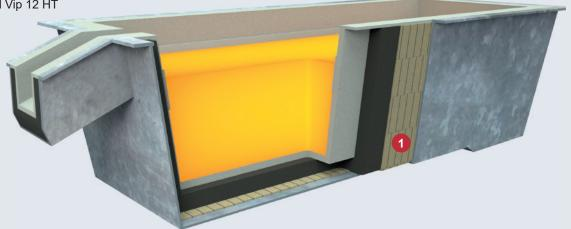
To protect the steel shell around the tundish and obtain the right temperature for steel prior to casting, the tundish is lined by refractory and insulating materials. The preferred insulating materials must be able to resist the high intermediate temperatures in the tundish and a relatively high compressive force.
